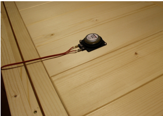
Fig. 47: Installation of the exciter
